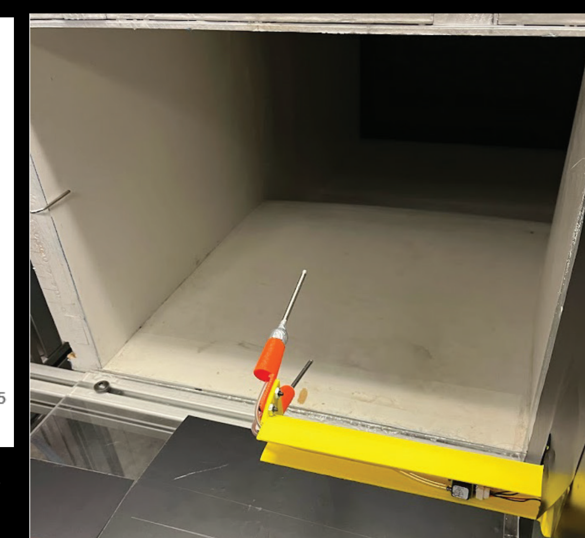
Dual pitot-static tube test with only stagnation ports connected.
