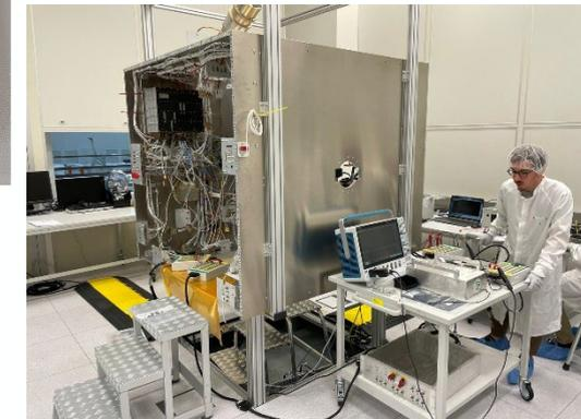
LSIB + Cubesats EM testing at OHB Hera Platform Avionics Test Bench (ATB)
