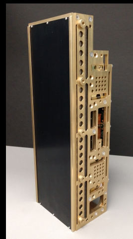
Mini-NS: Compact neutron and gamma-ray spectrometer for small spacecraft*
