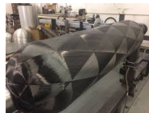
Filament-wound Propellant Tanks with 3D printed fittings
