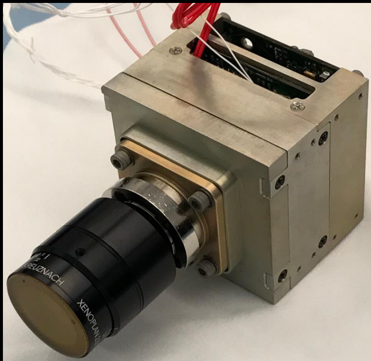
NEA Scout flight camera, based on Orbital Carbon Observatory 3 (OCO-3) mission context camera.
