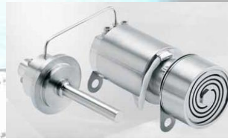
COTS AFRL developed AIM SX030 microcryocooler with cold finger to maintain detector at \leq 115K and iris controller
