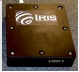
COTS AFRL developed AIM SX030 microcryocooler with cold finger to maintain detector at \leq 115K and iris controller
